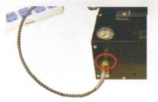
3. After connect the air outlet to the filling hose connector. We need to double check again these 3 connectors. Like spray soapy water to these adaptors to see if it has air leaking when air charging. We also can use very soft tissue close it to see if the tissue is swaying by the high pressure air. Fasten it when we see the bubbles or swaying tissues.
