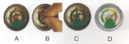
1= Fill Pressure Adjustment (Desired pressure pointer)
