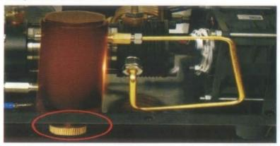
4. Locate the lubrication hole on the left hand side of the unit. Using the included oil applicator bottle, apply 2–3 drops of silicone oil every 5 fills or 1.5 hours of use (whichever comes first).
