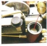
Drain the waste oil and water from oil drain valve every time to make sure compressor not in load status.
